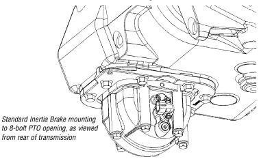
**Note:** Clean and remove all old gasket material from the mating surfaces of the inertia brake and transmission PTO coverings. Locate the harness push-in anchor point for reference during re-installation to 6-bolt opening.
