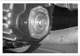
**5.** NOTE: Be sure that there is adequate transmission driveshaft/yoke clearance to the PTO before proceeding. If main vehicle driveline series is too large for the installation then this PTO cannot be used.
