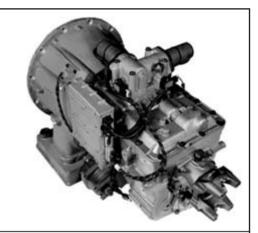
2. The Muncie RS4S-P86EM-A1CX PTO is designed to mount to the rear countershaft opening located directly below the rear output shaft of the transmission. Refer to the PTO owner's manual IN84-03 for applying safety labels and for installation procedures not shown here.
