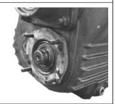
**4.** Shown is rear countershaft bearing exposed. **Do NOT install** PTO without the PTO adapter.
