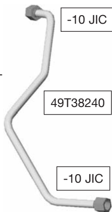
Pump Pressure Line
