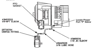
The hydraulic oil to engage the CLUTCH SHIFT PTO is supplied by transmission main pressure tap. This is the same port used to connect the CD Series lubrication line. The location of the tap is shown at Main Pressure Port "P" in the following diagram.
