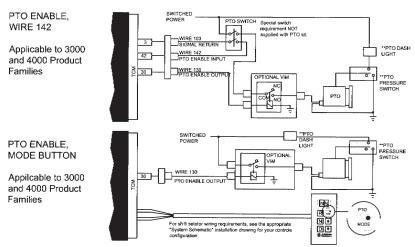
\*\* PTO switch, pressure switch, and dash are supplied with PTO activation kit included in Muncie PTOs.
