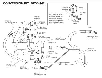
This kit is used to convert the standard built-in solenoid valve to a remote type without the replacement of the PTO end cover.
