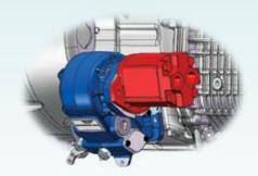
"T" Option - SAE A 2-Bolt 3.25" Pilot - 3/4" 11T Spline 3/8-16UNC-2B on 4.18" B.C.
