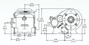
1-Assembly Arrangement with Muncie PKS Series pump mounted to front of PTO. Pump rotation - CW
